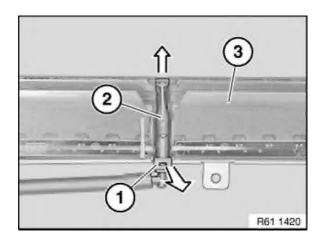
Unlock catch (1) and pull spray nozzle (2) in direction of arrow out of additional stop light (3).
