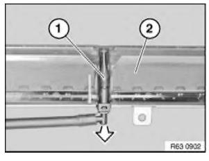
Remove spray nozzle (1) from rear spoiler (2) in direction of arrow.
